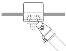
**SIZE** - 1/2" x 1 1/4" bolt. MATERIAL - Carbon Steel. FINISH - Plain or E.G. PATENT - No. 6,334,285 LISTING/APPROVAL -
