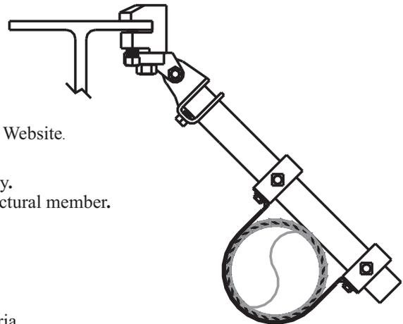
**FUNCTION** - Sway brace adapter for an *AFCON* sway brace assembly.
